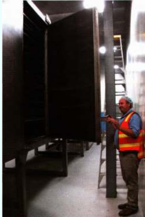
The pistachio oven is an Incus dry roaster capable of roasting 1200kg/ hour.
