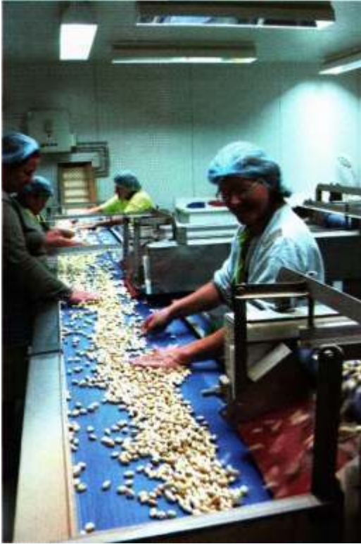
Hand inspection removes product defects
