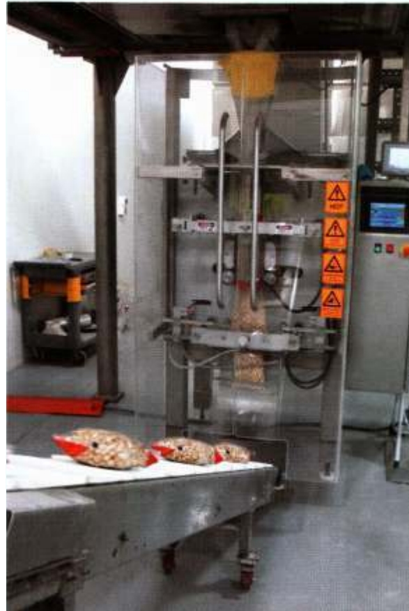
Packaging the product. Auto pack form fill machine is capable of bagging 35 x 900gram bags / min.
